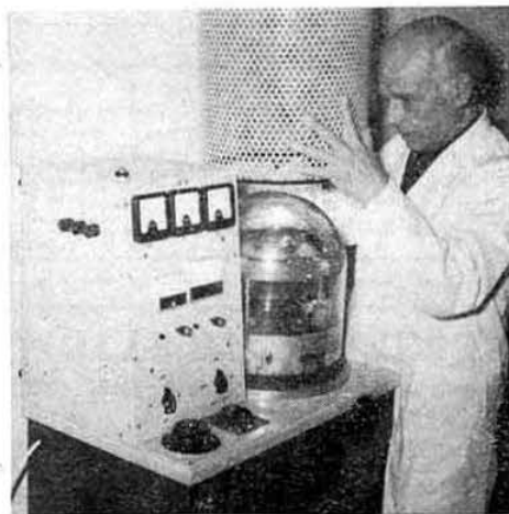
ABOVE: A SENATOR technician has loaded a batch of quartz plates into the ion-bombardment plant and is lowering the implosion safety-guard. Ion-bombardment removes microscopic deposits which may be difficult to remove by conventional chemical cleaning. Quartz crystals treated in this way possess superior ageing characteristics.
